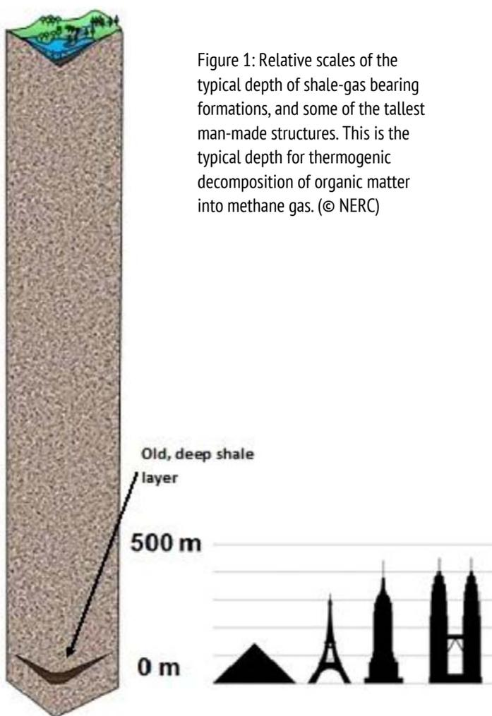
Figure 1: Relative scales of the typical depth of shale-gas bearing formations, and some of the tallest man-made structures. This is the typical depth for thermogenic decomposition of organic matter into methane gas. (© NERC)
