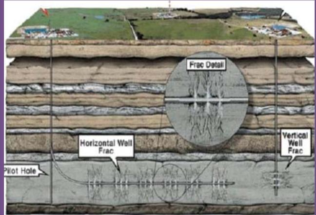
Figure 2: Schematic representation of shale gas operations. Most shale gas plays are at 2km to 5km depth, with drinking water aquifers within the first few hundred metres below the surface. Not to scale. (© B J Services)
