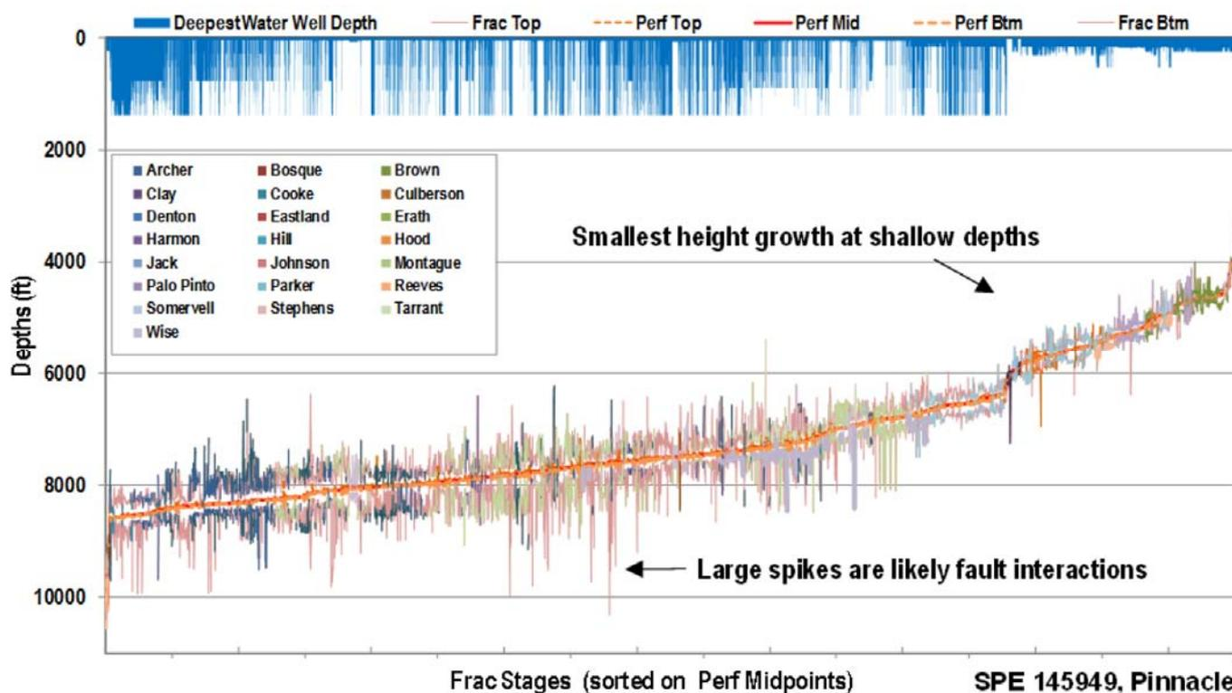
Figure 3: Data from the Barnett Shale (Texas, USA), obtained by Halliburton. Spikes represent fracture propagation depths. The tallest spikes are associated with fault linkage and propagation through pre-existing planes of mechanical weakness. The trend shows that with increasing depth, fracture magnitude increases, as a direct function of the increasing tensile strength of rocks with depth due to increasing pressure. (From Fisher, K., & Warpinski, N. 2011<sup>2</sup>)
