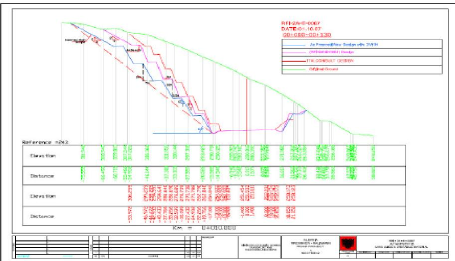
Bridge 1 CH18+800 Section 1. Typical Section through cut slope showing a succession of different design profiles. Figure is part of RFI 2A E 0067 dated 1 October 20008.
