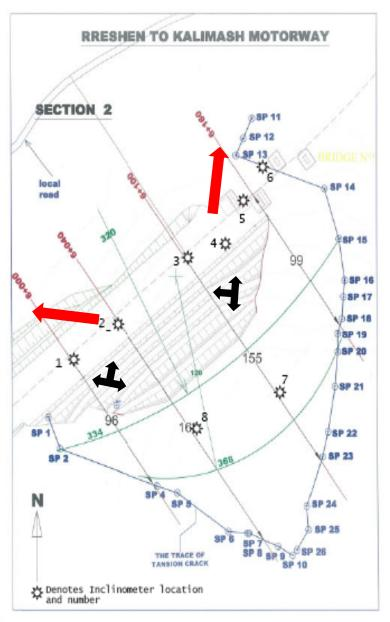
Section 2 Bridge 5. Survey of main scarp (TANSION CRACK on drawing) made by BEJV in March 2008. Inclinometer survey positions also shown.
