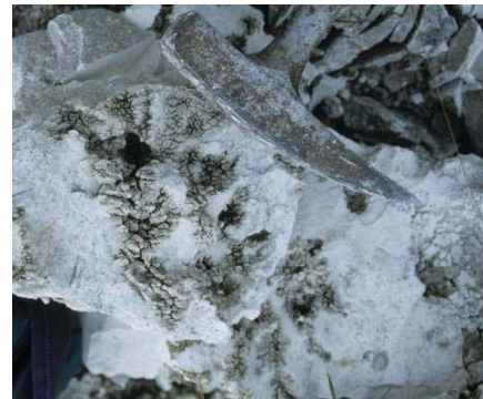
Tubular karst structures developed above a sheet flint band in the Chalk.
