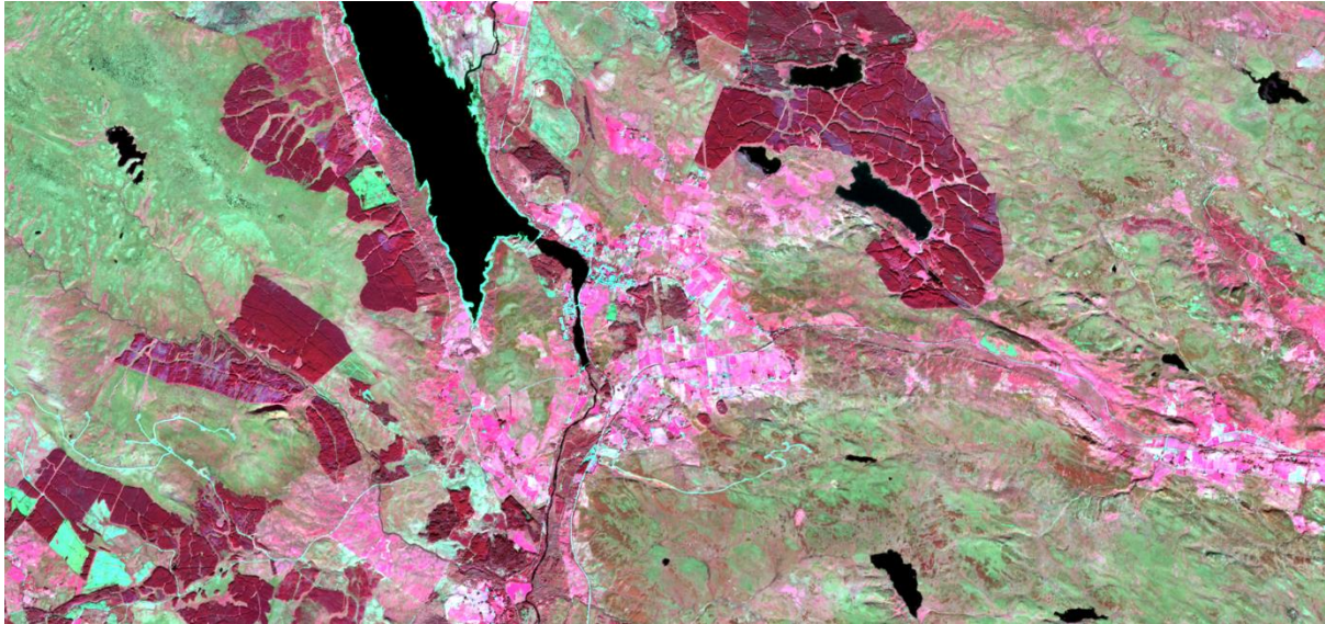
Sentinel 2 false colour infrared remotely sensed image utilised for detecting areas of peat for overhead line tower sites. Courtesy of David Giles
