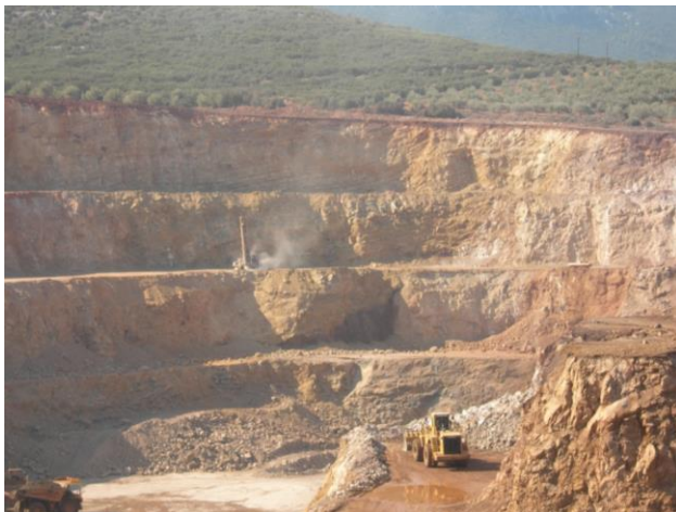
Figure 22: Modern open-pit mining of iron-nickel laterite employing sophisticated blasting technology, large haulage trucks and Doppler radar systems to monitor slope stability, Agios Ioannis mines at Neo Kokkino, Larymna, Greece. Photo: A. Demetriades
