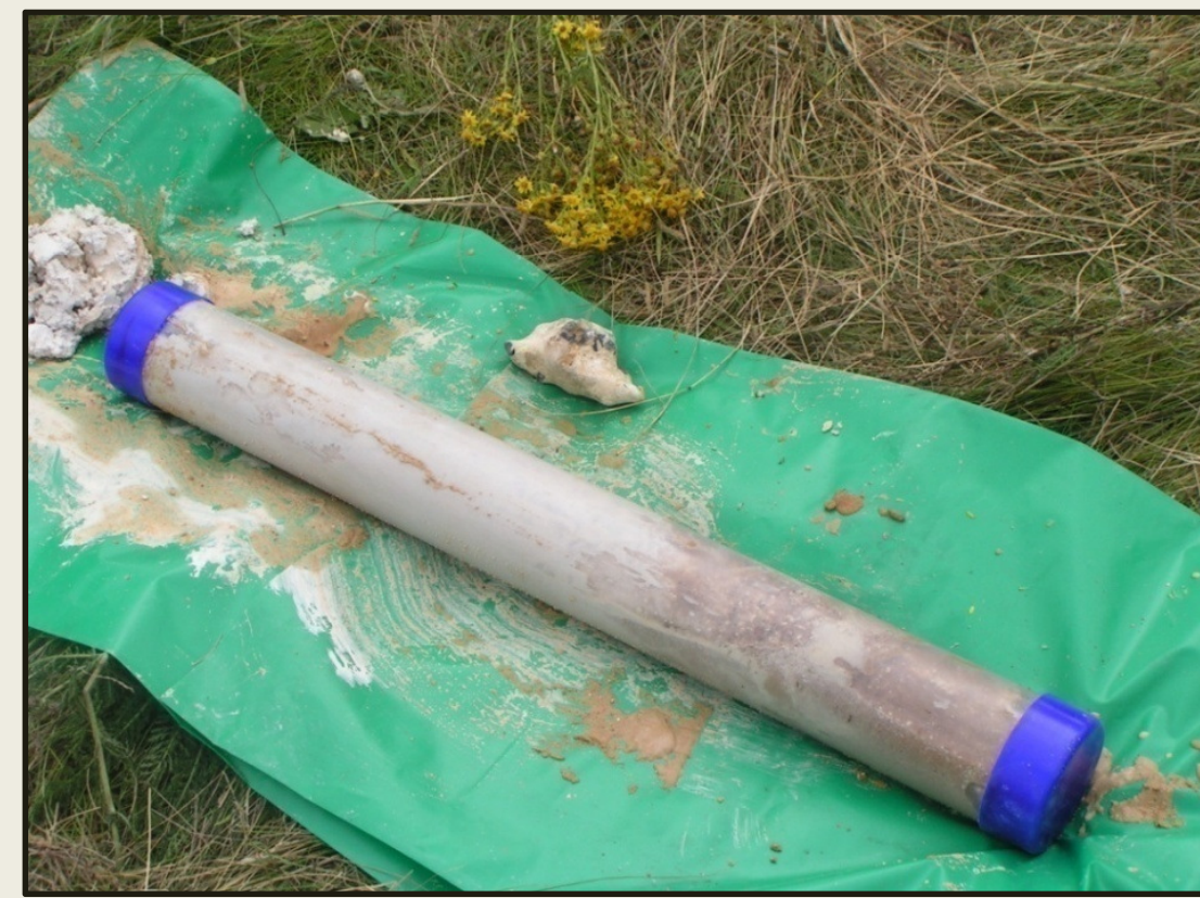
1 m x 0.1 m core samples removed from 10 m depth and 2 L of groundwater collected
