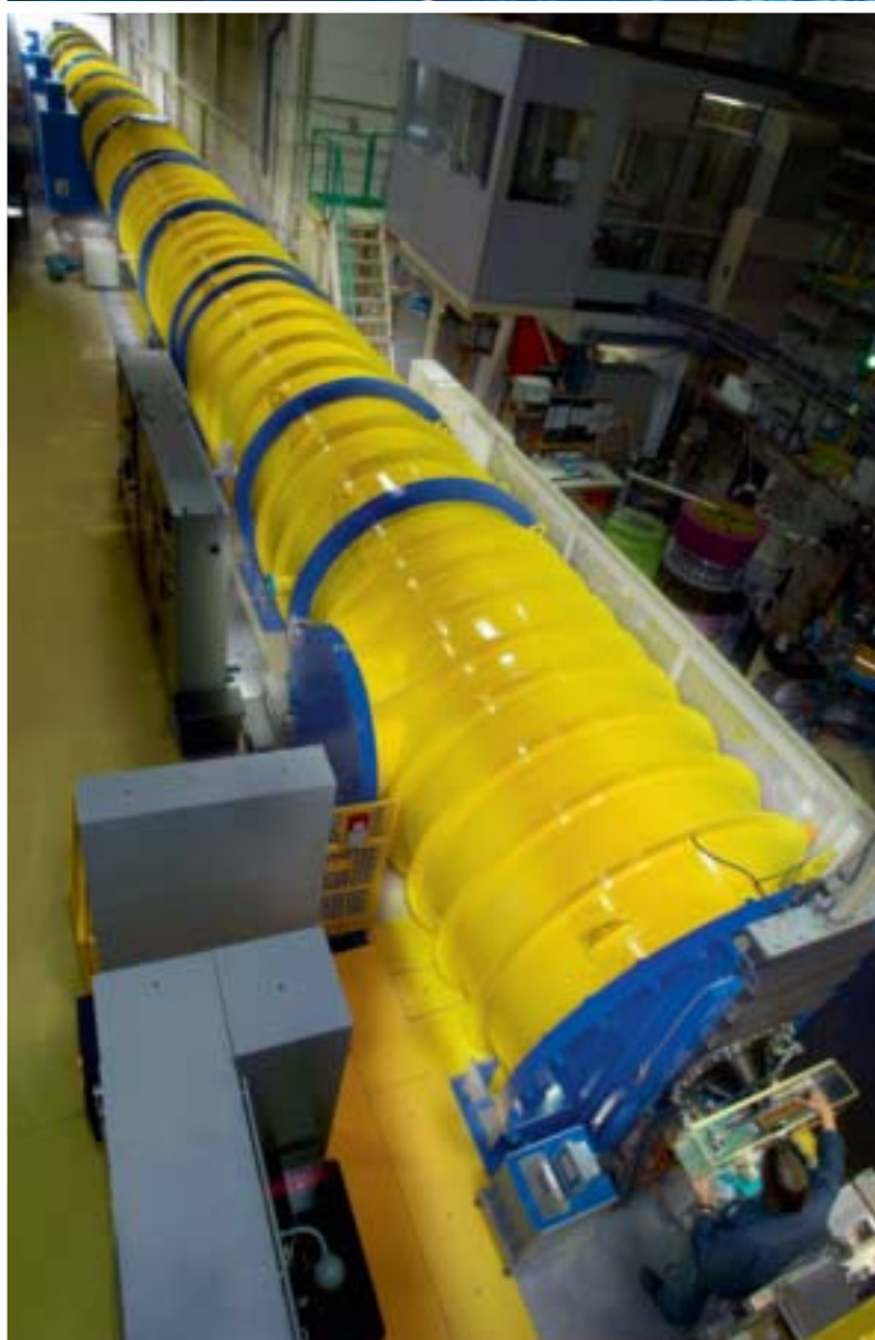
One of the beamlines at the ILL where neutrons are fired at samples to investigate their structure under a wide range of temperature and pressures
