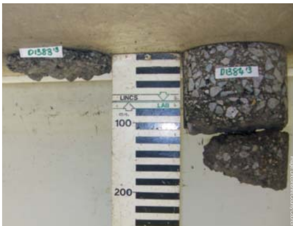
Varying depths of tarmacadam after coring investigation at Mole Drove
